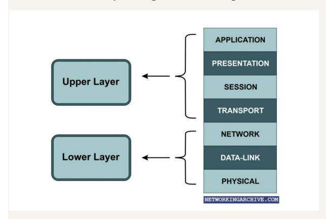
The International Organization for Standardization (ISO) developed the OSI reference model in 1984. It provides the standard of how traffic runs across the network.
